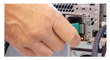
**7** Grasp the handle and pull the power supply out of the slot.
