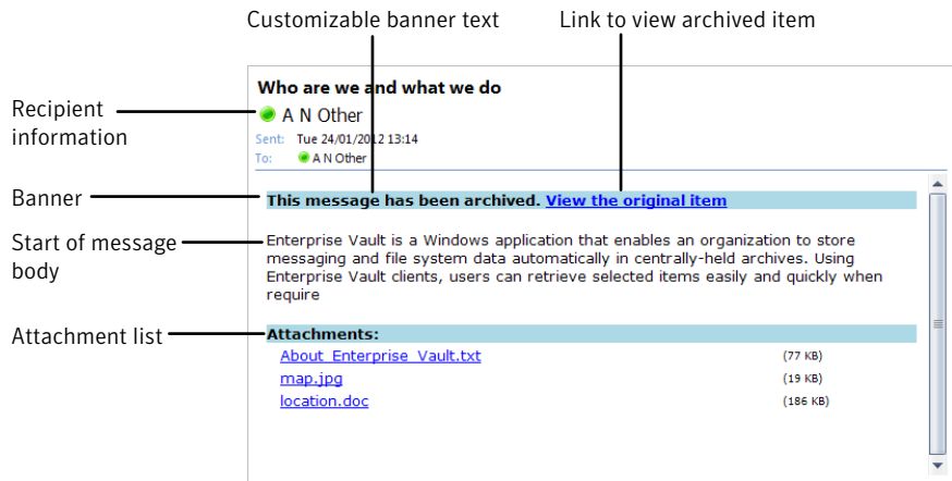
Figure 3-1 Structure of a shortcut
