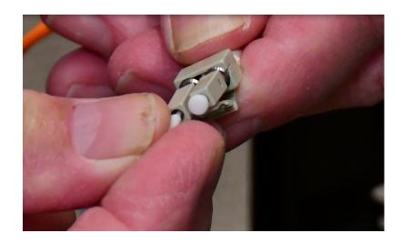
4 Remove the module by grasping the hinged removal tab at the front of the module.
