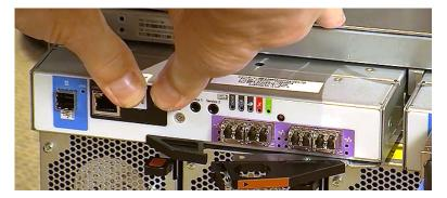
**3** Connect the cables to the replacement RAID Controller.
