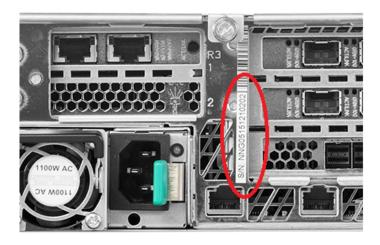
• For the 3360/5360 Appliance, the serial number is located on the rear panel of the appliance above PSU 1 and begins with letters VTAS.
