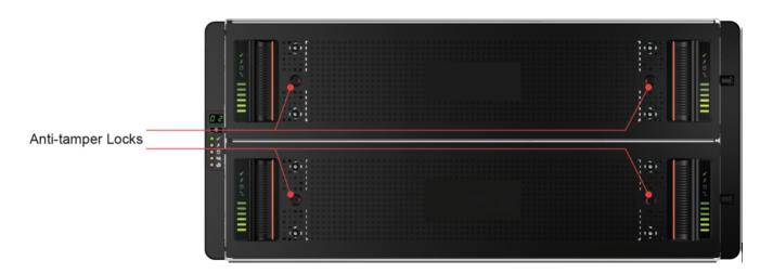
Unlock them if necessary by rotating them counterclockwise using a screwdriver with a Torx T20 bit.
