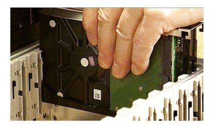
**Caution:** Damage can occur to a drive if it is removed while it is still spinning. Make sure that the drive has stopped prior to removal. Swap one drive at a time only. Removing more than one drive at one time can affect system functionality.
