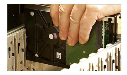
**3** Push the drive downwards and hold it down while sliding the drive carrier plate. This locks the drive in place.
