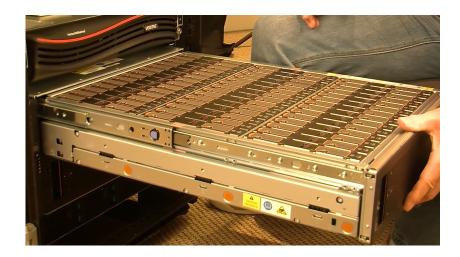
**Caution:** The drawer must not be left open for more than two minutes while the enclosure is powered.
