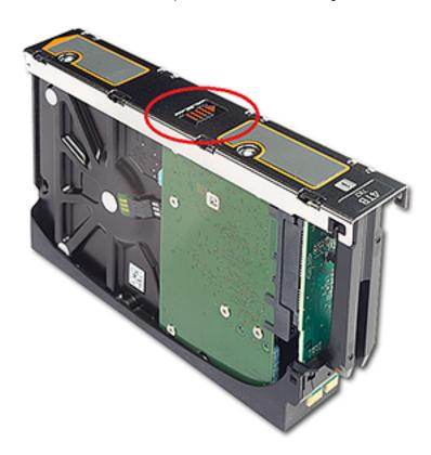
7 Lift the drive out of the slot approximately 1 inch (25mm), and then wait 30 seconds, allowing the drive to spin down.
