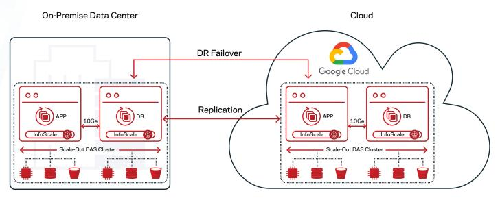
Figure 12. A sample InfoScale hybrid-cloud design concept.
