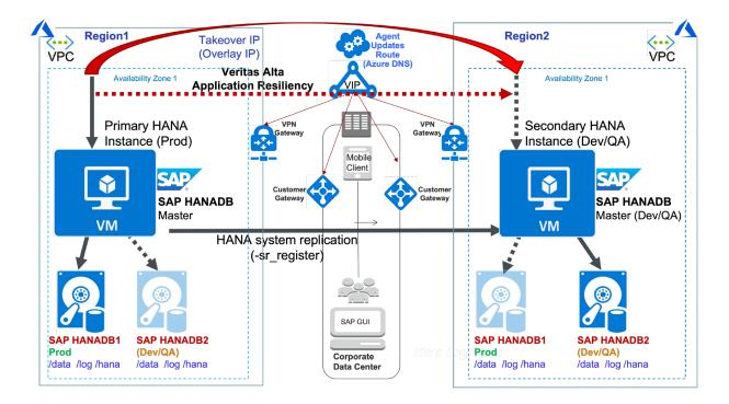
If the primary instance fails or becomes unavailable, the SAPHDB agent identifies the fault and automatically triggers the takeover operation on the secondary instance in the other region. The following graphic depicts this action:
