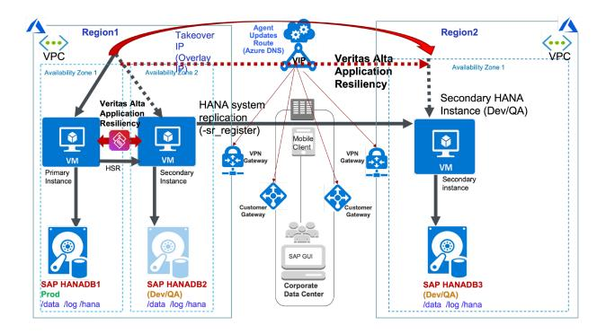
If the primary instance fails, the SAPHDB agent automatically triggers the takeover by failing over the IP resource from the primary to the secondary instance in the same region. Virtual IP failover operations are managed by the AZUREIP and the IP agents. The following graphic depicts how the secondary becomes the primary and is active in AvailabilityZone2:
