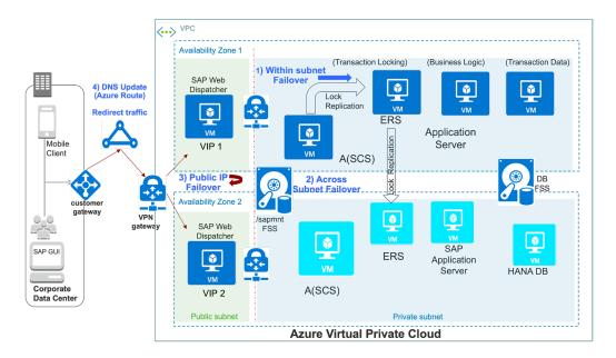
In addition to configuring SAP HANA for HA, DR, or both, you need to ensure that the client applications (for example, the S/4HANA/ NetWeaver application server, JDBC, ODBC connection, and so on) can re-establish their connection with the SAP HANA system after the failover. To do so, you can configure either network-based IP redirection or network-based DNS redirection of your SAP HANA system. Veritas agents for SAP support end-to-end HA and DR for SAP NetWeaver and SAP S/4HANA as well.
