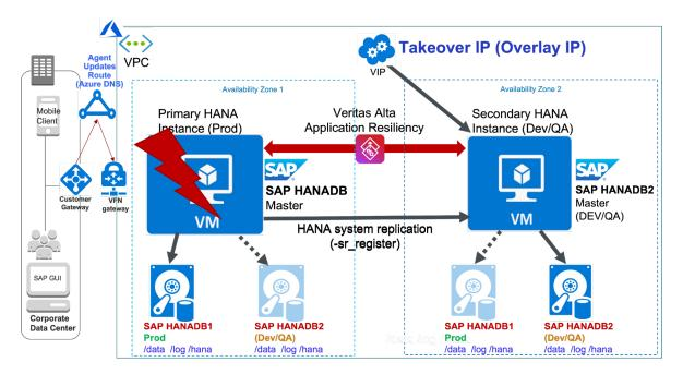
You may choose to clear the fault and perform any other necessary maintenance activities on the old primary instance. Thereafter, the SAPHDB agent can automatically designate it as the secondary instance by using the auto re-register feature. HANA System Replication can then continue the data replication in the reverse direction. The following graphic depicts this action:
