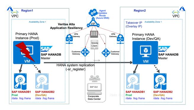
You'll need to clear the fault and perform any other necessary maintenance activities on the old primary instance. Thereafter, the SAPHDB agent automatically designates it as the secondary instance by using the auto re-register feature. The following graphic depicts this action:
