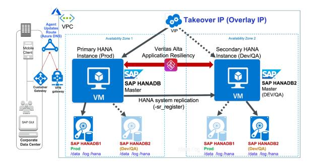
If the primary instance fails or becomes unavailable, the SAPHDB agent identifies the fault and automatically triggers the takeover operation on the secondary instance. The following graphic depicts this action:
