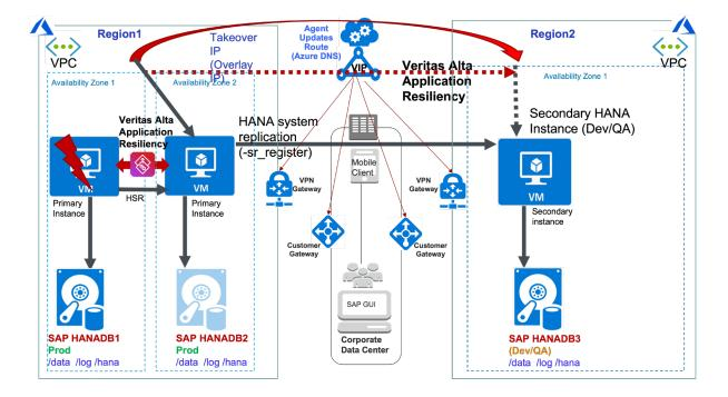
If all the instances within in an AZ or a region fail, the SAPHDB agent automatically triggers the takeover action by failing over the IP resource from the primary to the secondary instance in the remote region. The following graphic depicts how the secondary in the remote region becomes the primary:
