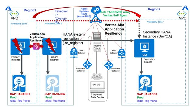
Thereafter, you'll need to clear the faults on the instances in the Region1 and re-register them with the current primary in Region2. The following graphic shows the direction of the replication being reversed:
