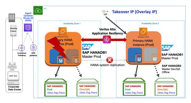
You may choose to clear the fault and perform any other necessary maintenance activities on the old primary instance. The SAPHDB agent can then automatically designate the original primary instance as the secondary instance by using the auto re-register feature. HANA System Replication will then continue the data replication in the reverse direction. This is shown in the following graphic:
