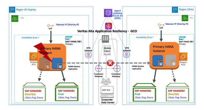
You'll need to clear the fault and perform any other necessary maintenance activities on the old primary instance. The SAPHDB agent can then automatically designate the original primary instance as the secondary instance by using the auto re-register feature. The is shown in the following graphic:
