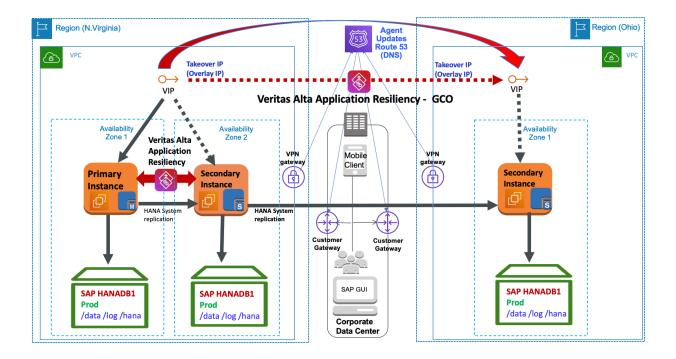
If the primary instance fails, the SAPHDB agent automatically triggers the takeover by failing over the IP resource from the primary to the secondary instance in the same region. Virtual IP failover operations are managed by the AWSIP and the IP agents. The following graphic shows how the secondary becomes the primary and is active in AvailabilityZone2:
