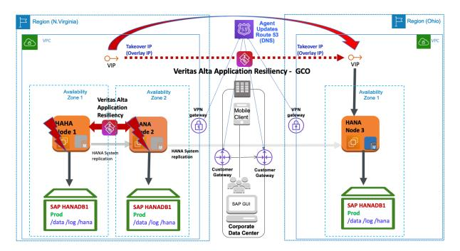
Thereafter, you'll need to clear the faults on the instances in the N.Virginia region and re-register them with the current primary in Ohio. The following graphic shows the direction of the replication being reversed:
