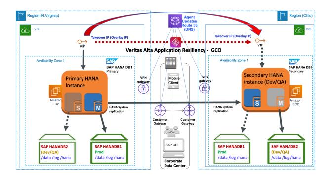
If the primary instance fails or becomes unavailable, the SAPHDB agent identifies the fault and automatically triggers the takeover operation on the secondary instance in the other region. The is shown in the following graphic:
