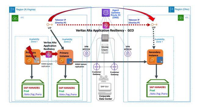
If all the instances within in an AZ or a region fail, the SAPHDB agent automatically triggers the takeover action by failing over the IP resource from the primary to the secondary instance in the remote region. This is shown in the following graphic where the secondary in the remote region becomes the primary:
