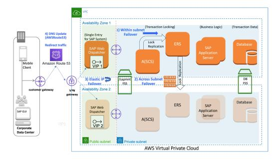
In addition to configuring SAP HANA for HA, DR, or both HA and DR, you need to ensure that the client applications (i.e. the S/4HANA/ NetWeaver application server, JDBC, ODBC connection, and so on) can re-establish their connection with the SAP HANA database after the failover. To do so, you can configure either network-based IP redirection or network-based DNS redirection of your SAP HANA system. The Veritas agents for SAP support end-to-end HA and DR for SAP NetWeaver and SAP S/4HANA.
