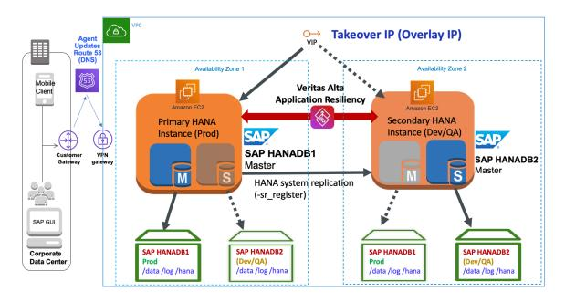
If the primary instance fails or becomes unavailable, the SAPHDB agent identifies the fault and automatically triggers the takeover operation on the secondary instance. This is shown in the following graphic:
