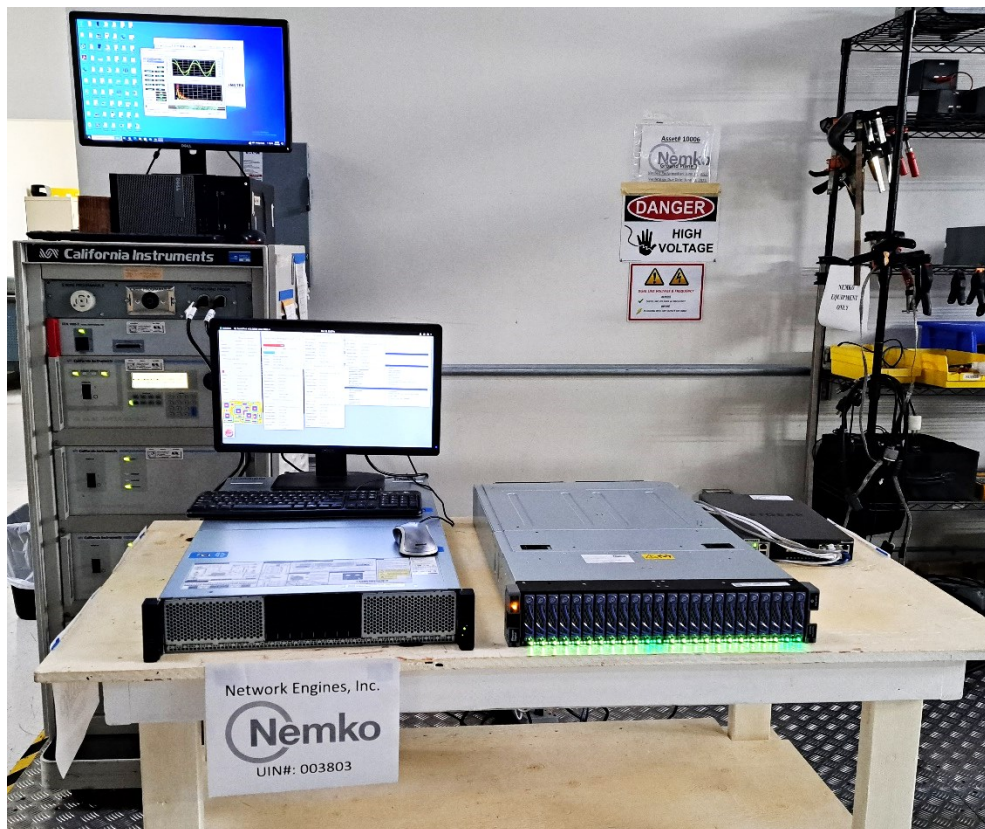
Figure 8.4-1: Conducted emissions – Harmonic current emissions setup photo
