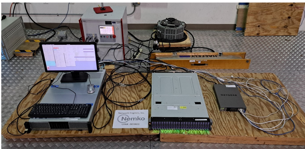
Figure 9.5-1: Fast transients on AC Mains setup photo
