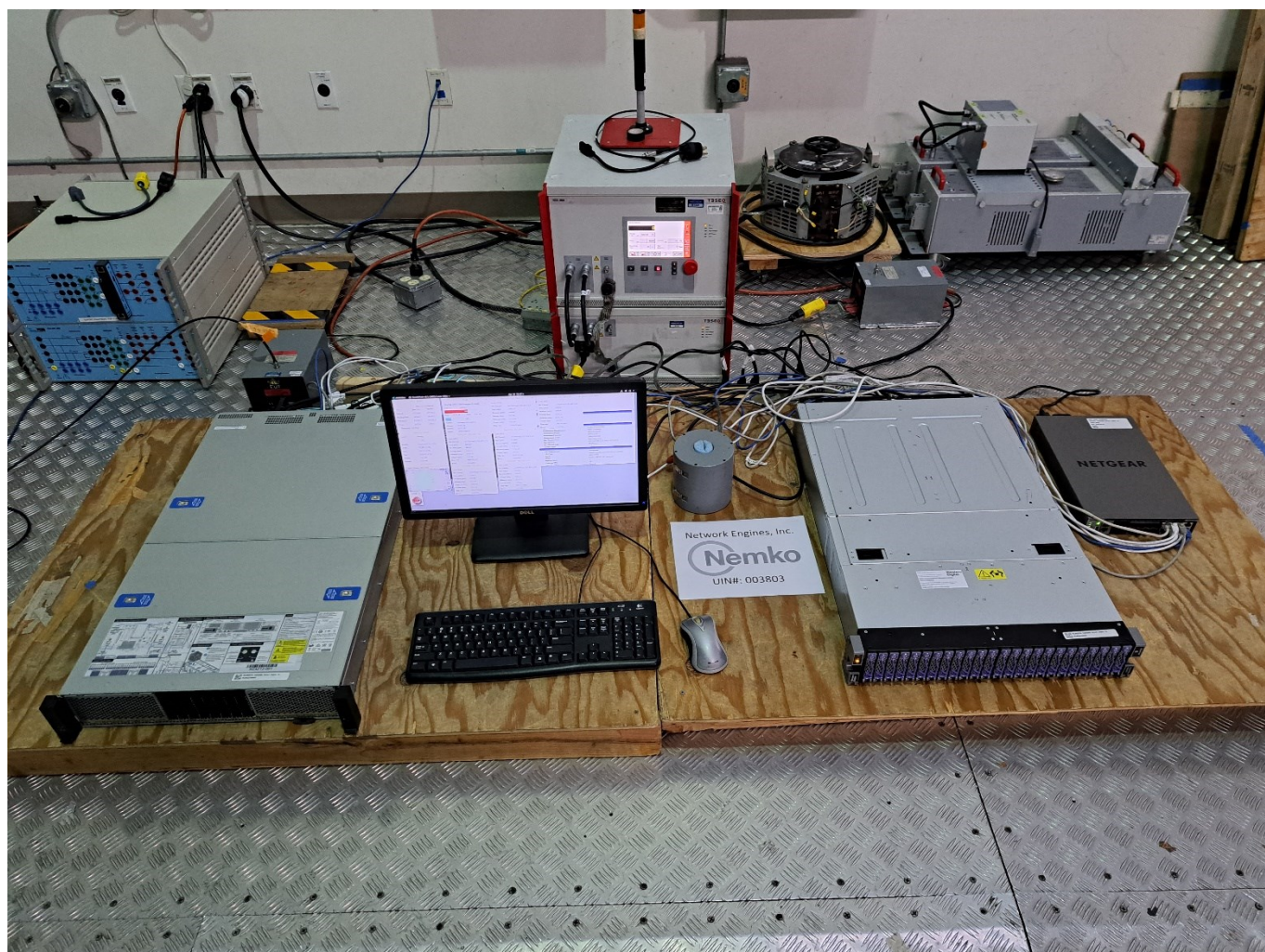
Figure 9.2-2: Radio-frequency continuous conducted on I/O cable setup photo
