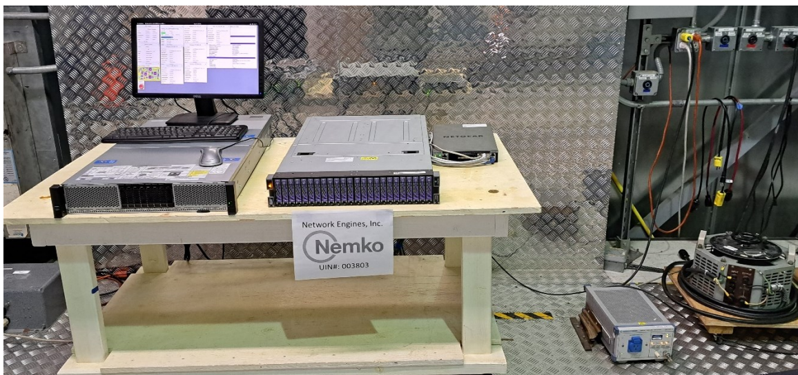
Figure 8.3-3: Conducted emissions – Asymmetric mode setup photo
