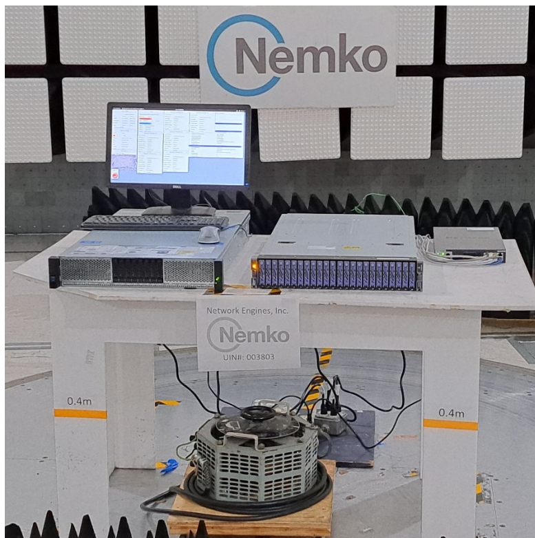
Figure 8.1-5: Radiated emissions setup photo above 1 GHz
