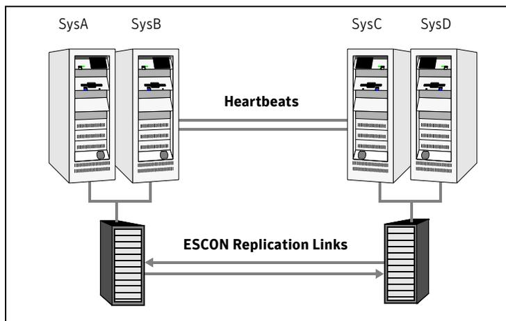
This example depicts a sample configuration where SysA and SysB are in one system zone, and SysC and SysD are in another system zone. Use the SystemZone attribute to create these zones.
