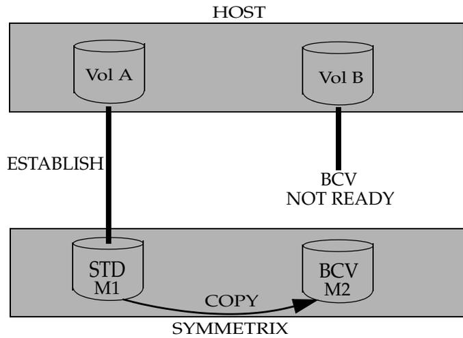
Symmetrix internal functions create the appropriate mirror relationships and copy data from the standard to the BCV devices. The BCV disk group is synchronized when the standard device mirrors and the BCV mirrors contain identical data. To use a BCV disk group for business continuance procedures, the BCV disk group must be split to make the BCV disk group and volumes available to the host.
