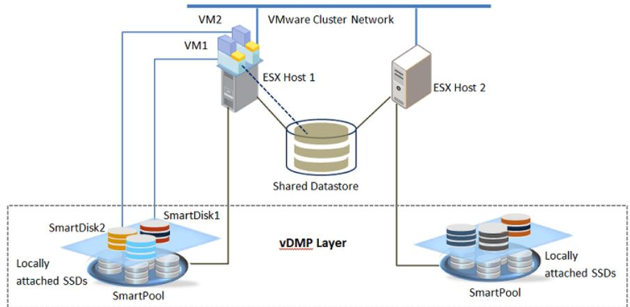
After vMotion, the first I/O to the cache area fails and the request is forwarded to the back-end storage (data disks). SFW considers the I/O failure as a vMotion event and informs the VxDMP layer to allocate a SmartDisk of the required capacity. After the VxDMP layer allocates a SmartDisk, SFW retrieves the cache area details from the registry and creates a similar cache area on the SmartDisk that is assigned to the virtual machine after vMotion.
