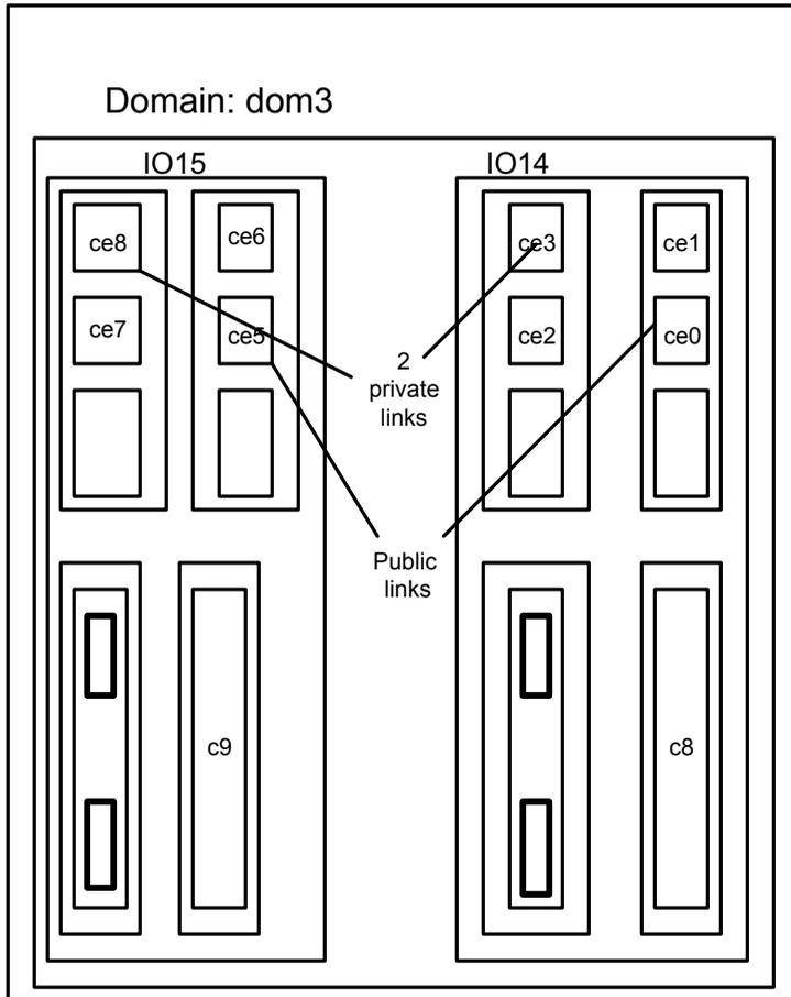
For e12K/15K/25K: In the following scenario, a cluster consists of the dom3 and the S6800f0 domains. The cluster is running service groups on the dom3 domain, which includes I/O boards IO14 and IO15. IO15 requires dynamic reconfiguration because of a malfunctioning component. The domain S6800f0 includes I/O boards IB8 and IB6. The disk controllers and NICs are labeled in the following diagrams.
