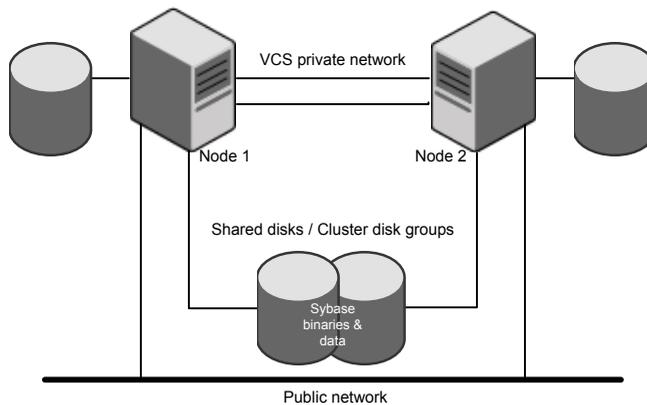
**Figure 1-2** illustrates a sample configuration in which Sybase binaries are installed locally on each node in the cluster and the Sybase data is on shared disks or shared cluster disk groups managed using VxVM.
