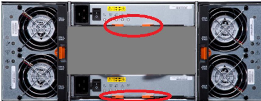
While removing the power canister, you might notice an increase in fan speed. The fan speed returns to normal after you have replaced the power canister.
