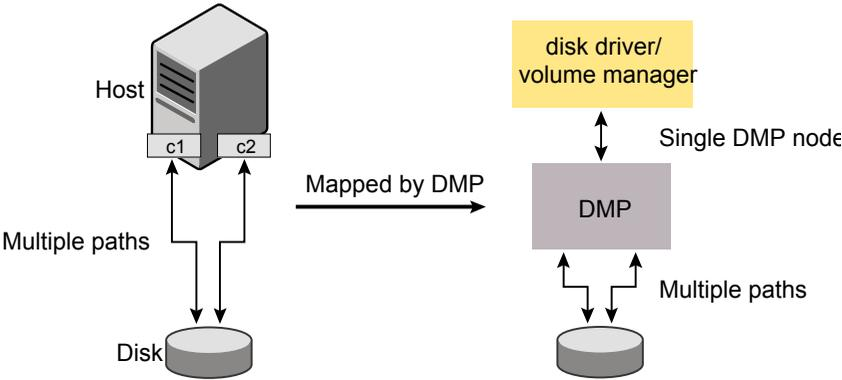
The following figure shows an example where two paths, c1t99d0 and c2t99d0, exist to a single disk in the enclosure, but the single DMP node, enc0\_0, is used to access it.
