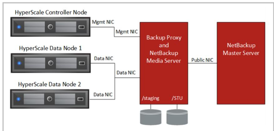
In addition, the NetBackup administrator must configure the directory path on which HyperScale backups are stored; this is known as the staging location. This location needs to be on a separate set of disks than that of the storage unit (STU) disks (in case of a hard-disk backed STU).
